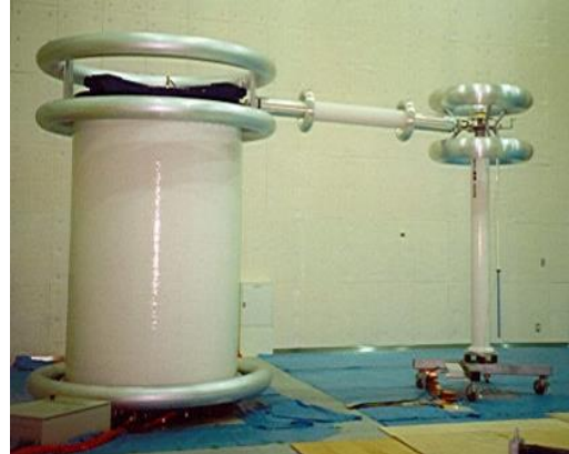
Test system 350 kV, 2 A with damping resistor
